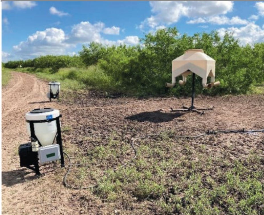
Figure 5. Sprayers with ground nozzles to treat white-tailed deer at corn feeders.
