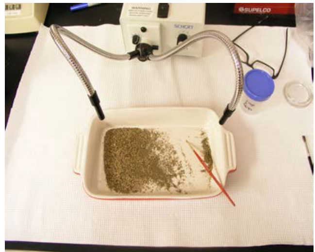
(Left) A No. 14 covered soil sieve for sorting bark. (Right) A white ceramic baking pan with sifted bark ready for viewing under a dissecting microscope.
