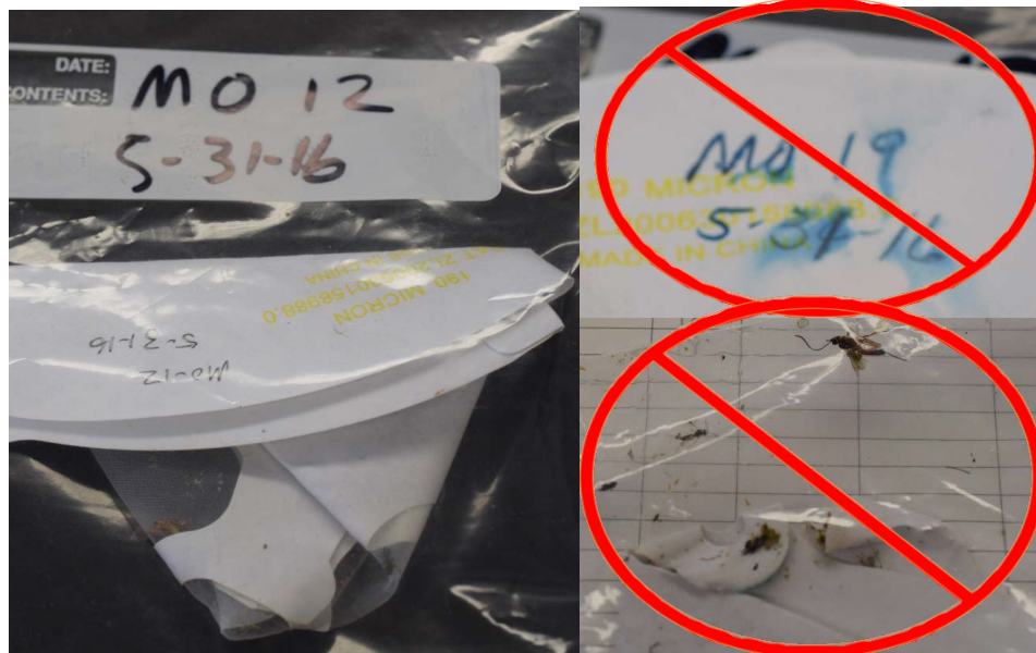
Label the filter paper in pencil (left) to avoid ink smearing (right). Fold the filter paper over (left) to avoid insects spilling out prior to processing (right).
