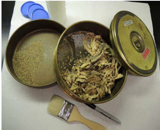
(Left) A No. 14 covered soil sieve for sorting bark. (Right) A white ceramic baking pan with sifted bark ready for viewing under a dissecting microscope.
